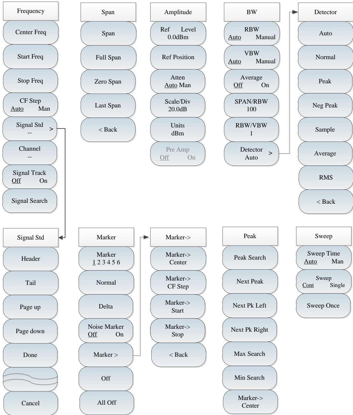
Fig. 5-3 Overall Block Diagram of Interference Analyzer Menu
