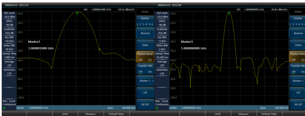
Fig 4-11 Noise measurement by using the noise marker function
